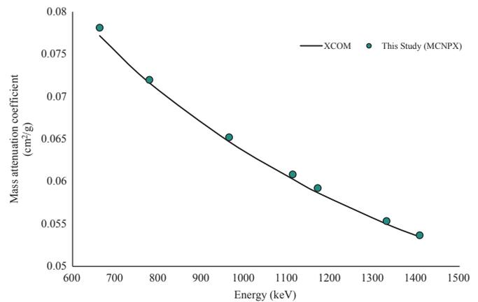
Fig. 3. MCNPX and XCOM data comparison for mass attenuation coefficients of concrete.
