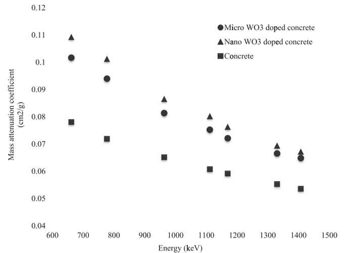
Fig. 4. Comparison of mass attenuation coefficients of concrete among pure concrete, micro-WO<sub>3</sub>, nano-WO<sub>3</sub> concrete.
